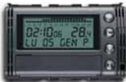
2CSE1201EL Summer/winter electronic programmable thermostat, with daily and weekly programming and 3 temperature levels. Output contact NO, 5A (AC1)/2A (AC15) – 250V~
