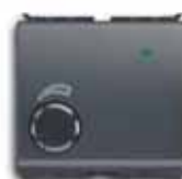
2CSE1209EL Electronic dimmer with push button control for resistive-inductive loads and electronic power supplies for very low voltage halogen bulbs, 25-300W (25-250VA), 230V~ 50/60Hz
