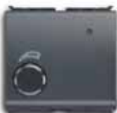
2CSE1206EL (1) Electronic dimmer with push button control for resistive and inductive loads, 60-500W (60-500VA), 230V~ 50/60Hz
