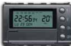
2CSE1203EL 2 channels daily/weekly electronic programmer with 2 change-over output contacts NO/NC, 5A (AC1)/2A (AC15) – 250V~
