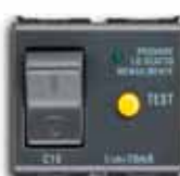
2CSE1309EL RCBO, 1P+N, C16 - 10mA, 3kA breaking capacity
