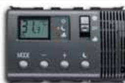
2CSE1202EL Summer/winter electronic thermostat, with night-time reduction remote control input and 3 temperature levels. Output contact NO, 5A (AC1)/2A (AC15) – 250V~
